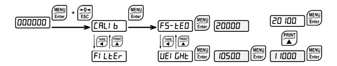
After having performed the **WEIGHT ZERO SET** procedure, it is possible to load a sample weight onto the weighing system, equal to the maximum quantity that is to be weighed or **at least the 50%** of it.
