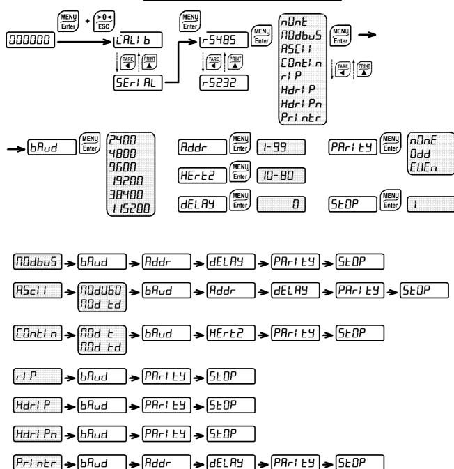
According to the protocol chosen (modbus, ascii...) only the necessary settings will be visualised in sequence (see above diagram).
