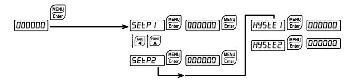
The LEDs light up in sequence and indicate that a setting is being visualised and not the weight. These values are set to zero if a new calibration is performed or the weight decimals are changed.
