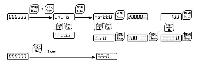
This menu may also be accessed directly from the visualisation of the weight holding down the ESC button for 3 seconds.
