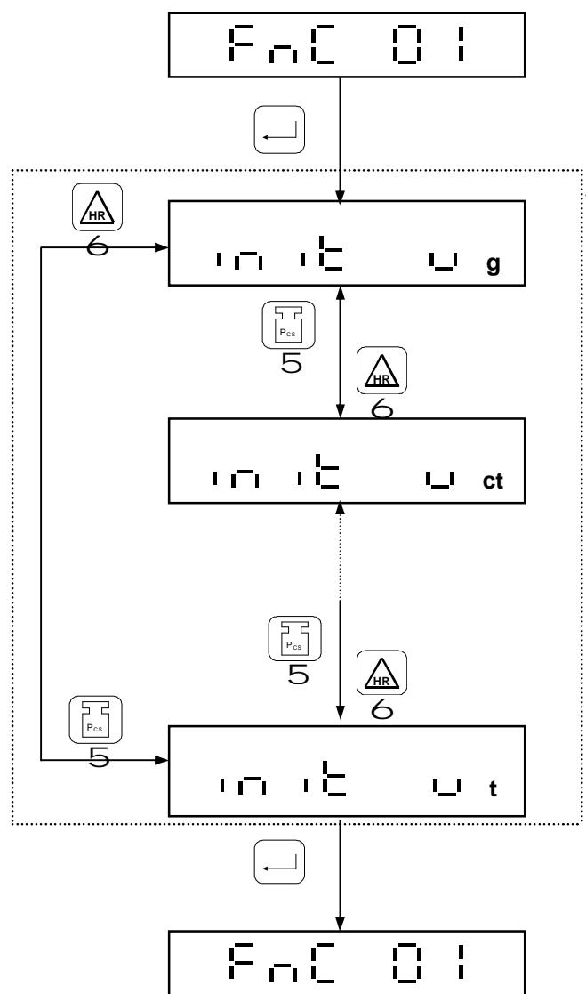
Use the or key to select the unit in cycle, and press the key to confirm the setting.
