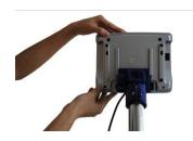
**Step 4**: After connecting load cell connector to load cell port, the installation is completed.
