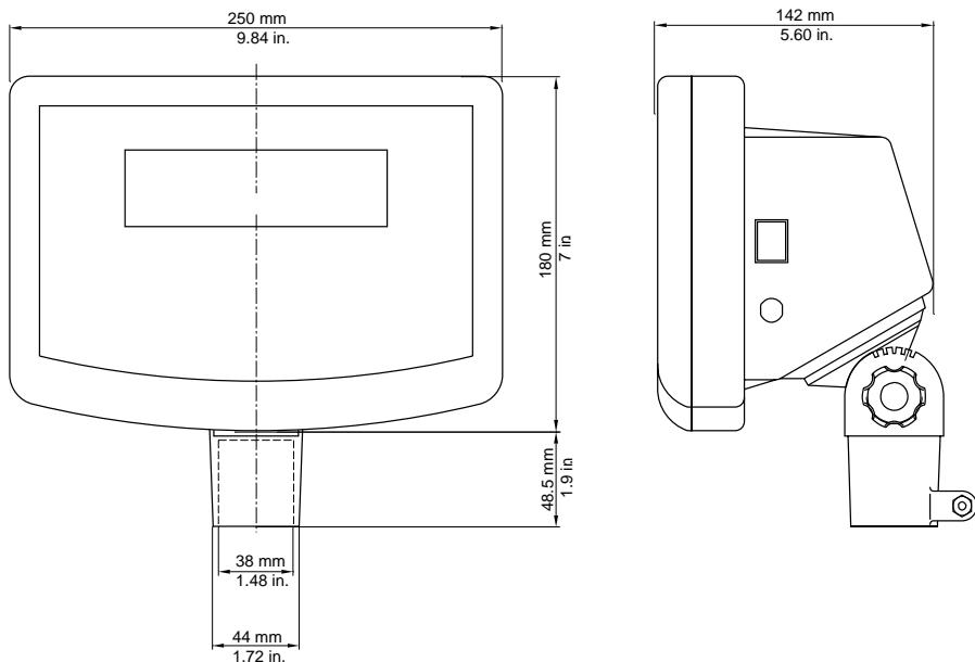
Figure 8-1. T21P Indicator Overall Dimensions.
