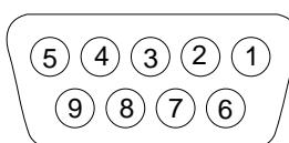
Figure 2-2. View of RS232 Pins on indicator. (Item 9 in Figure 1-1)
